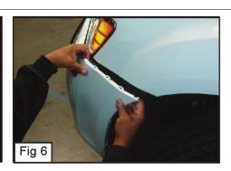
The instruction here is for your reference only. You may need to bend the billet grille bars or tabs a little bit to adjust to fit. We strongly recommend the professional installer for best result.
