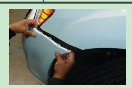
Step 2-5: Pull Side Fender outward to Unclip.
