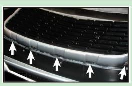
Step3-3:Remove 11 Clips around the Grille Shell.
