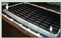
Step3-2:Remove 2 Screws on the corners of the Grille Shell.
