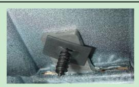
Step4-5: Place a #8 Flat Nut on the outer edge on the bracket and thread with a #8 Screw.
