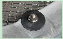
Step4-3:Insert Fender Flat washers along the top of the Screws on the mesh Grille, Tight with Lock Nuts.
