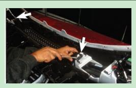
Step3-1: Remove 2 Clips on the Bumper Support.
