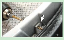
Step4-4:Drill a 3/16 Hole through the Brackets on the side and bottom of the Mesh Grill.
