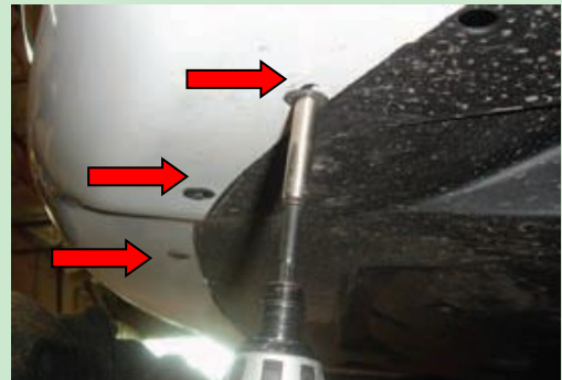
Step 2-4: Remove 7 Screws from Underneath of the Factory Front Bumper
