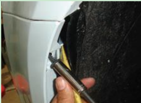
Step 2-3: Remove 10mm Bolt on the inner Fender
