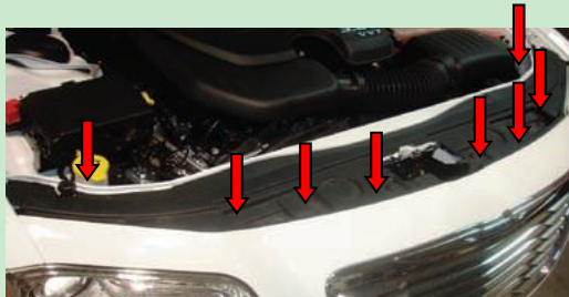
Step 2-1: Pop hood. Remove 8 clips on the Plastic Cover
