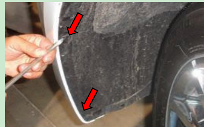
Step2-2: Remove 2 clips on side Fender Well
