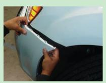
Step 3-5: Pull Side Fender outward to Unclip.
