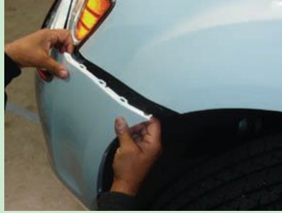
Step 3-5: Pull Side Fender outward to Unclip.
