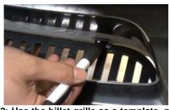
Step 4-2: Use the billet grille as a template, mark the location of the welded tab holes on the lip of bumper opening.
