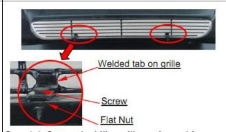
Step 4-3: Drill (2) holes on the lip of the Step 4-4: Center the billet grille again, and fasten the billet grille with the screws & flat nuts.
