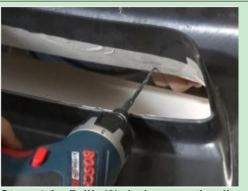
Step 4-3: Drill (2) holes on the lip of the Step 4-4: Center the billet grille again, and fasten bumper opening according to the marks
