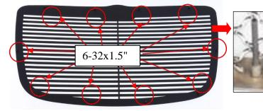
Center the grille into the opening on the factory front bumper. Be sure the studs are through the factory holes on the front bumper.
