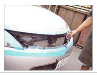
Once the lip is removed from the bumper it may be necessary to smooth out the rough edges left after cutting. Center the billet grille into the factory grille shell opening. Place the powder coated L-brackets over the fully threaded studs so that the L portion is hooked over the backside of the bumper and hold in place using the k-lock nuts. Attach the powder coated flat brackets to the upper mounts on the billet grille using the Allen head bolts and k-lock nuts.
