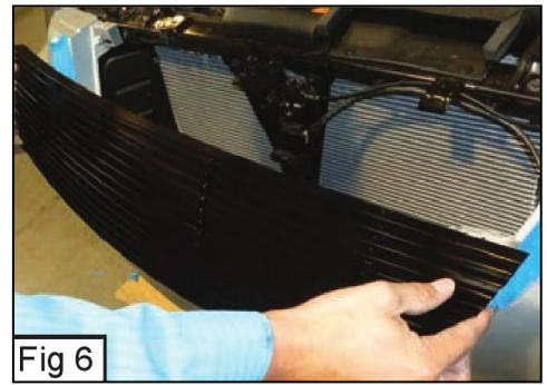
The instruction here is for your reference only. You may need to bend the billet grille bars or tabs a little bit to adjust to fit. We strongly recommend the professional installer for best result. Please use masking tape and tape the OEM grille shell along the edge to protect your vehicle during installation. We are not responsible for any damage caused by the installation. Thank you for choosing our product!
