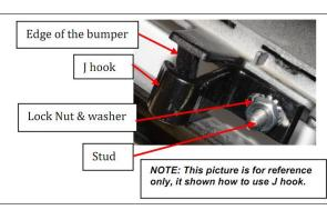
6 Re-install the plastic bumper shroud which was removed in step 2
