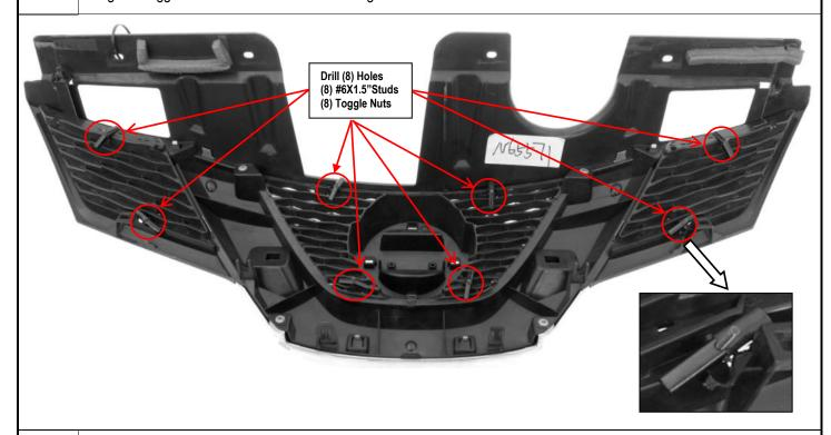
5 Make sure the insert is centered and tighten the hardware.
