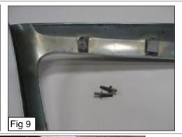
Thread a stud in each nut welded to the grille.
