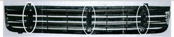
Figure 3 – Rear view of Brackets attached with Flange Nuts
