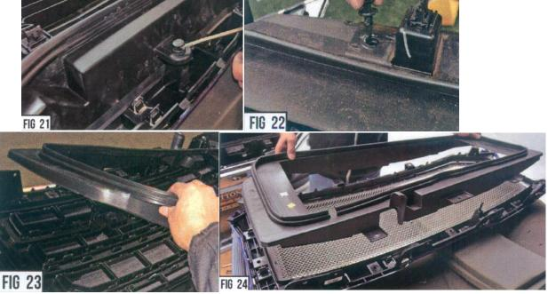
With the radiator shroud removed and safely out of the way. It is now time cut into the factory grille plastic pattern design and separate the factory grille shell to re-purpose and utilize with your new grille. From the grilles backside, make a proper cutting path using a paint pen or bright marker to highlight the correct cutting patch along the outer edge of the plastic grille pattern.
