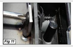
Your installation is now complete. Reattach the grille/ bumper assembly back to the vehicle in reverse order of removal. Use the included plastic rivets to replace the rivets removed in step 9. If you would wish to reuse your factory emblem please see page 5 for removal from the factory grille. Make sure you reconnect all disconnected wiring harness and reattach all clips and screws.
