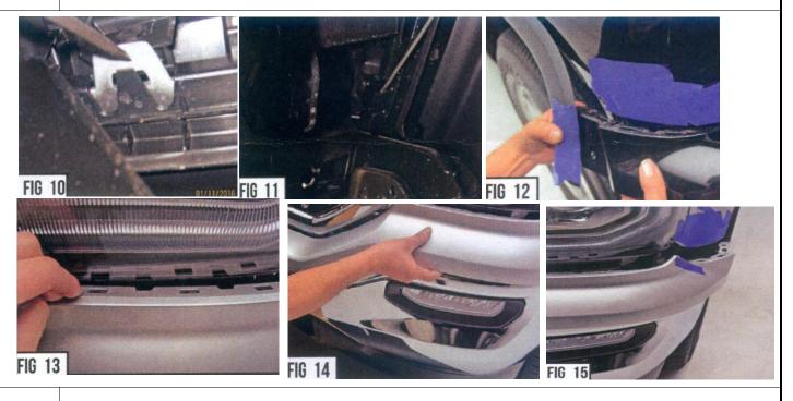
At this point, you need to remove the vehicles plastic lower bumper valance (a long and slim trim panel that is located directly above the front bumper, below the grille, and is usually color matched to the vehicle body color). Slip out the valance away from where it meets the front fender. You will need to unfasten several tabs that latch the whole piece from under and behind bumper and underneath headlights.
