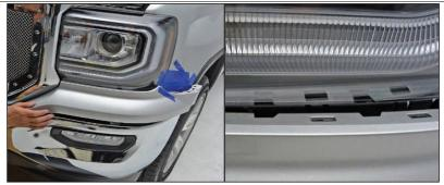
Put Core Support Cover back into place and fasten down with plastic push tabs that were removed prior. Re-Install all hardware that was removed in step #4.
