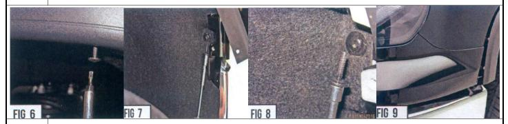
It is now time to loosen the vehicle wheel well fender trim. Start at the top middle, and working your way towards the very front of the fender trim where it meets the front bumper, use a torq bit remove screws. With the front half fender trim loose and pulled out of the way, (as seen in Figure 7) you can access the additional hardware that secure the plastic lower bumper valance. Remove these bolts and set aside all hardware for reinstallation later.
