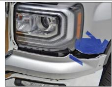
Carefully slip valance into place underneath headlights. Give it a firm press to get everything into position. Fit Valance up and mate it to front fender and finally slip fender trim back over each piece so it all fits nice and tight.
