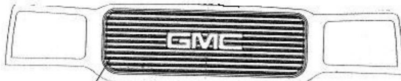
Cut and remove stock grille work a 1/4" reveal behind chrome ring and sad smooth
