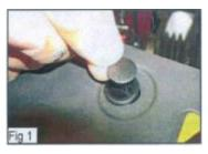
1. Identify the grille & hardware with parts 2. Start of by removing the twelve plastic pop clips along the top of the radiator cover using flat screw driver (Fig 1).
