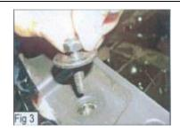
4.Remove the four 10mm bolts located along the top of the factory grill (Fig 3).
