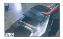
secure the air vent plastic to the factory looking at the front side, insert the billet parts bag, locate the small square tabs on grille, the bolts from the factory grille will grille into the opening in the factory grille (Fig 22).
