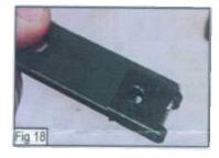
17. Take the black plastic back section of the factory grill and the grille shell and reassemble them into one section, just the same way they were before you separated them. Take the seven extension brackets and install the u-nuts onto them as in (Fig 18). The u-nuts install onto the end of the extension bracket that has the elongated hole, push the u-nut all the way onto the bracket.
