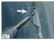
7. Now using a T15 torx bit remove two 8.Pull back the fender trim and remove one torx bolts from the top and front edges of 7mm bolt from the front of both front fenderwells (Fig 7) located just behind where you removed the forward torx bolts.
