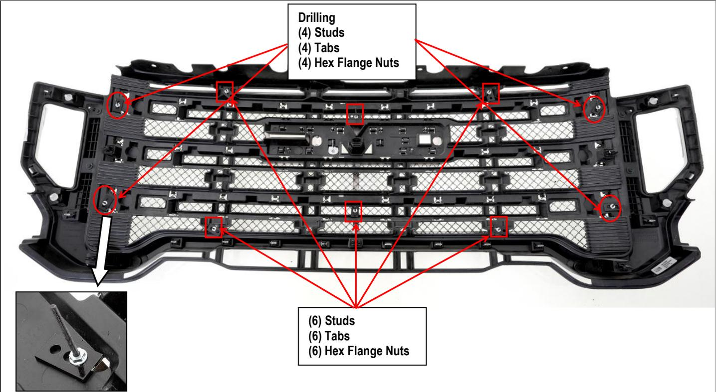
**6** Make sure the insert is centered and tighten the hardware.
