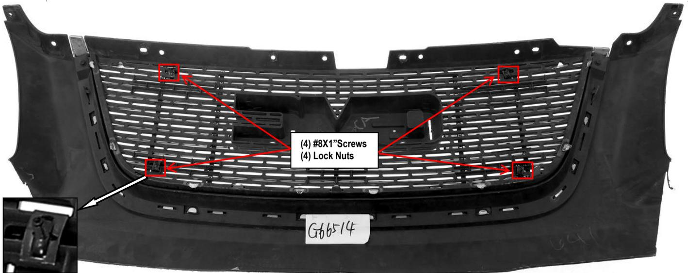
4 Make sure the insert is centered and tighten the hardware.
