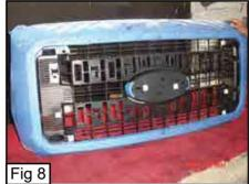
Now you need to cut out the inner section of the black grille section. You will cut around the inner edge of the black section as marked in (Fig 9). The 4 corner areas and the right and left sides will not be cut out, make sure to leave the areas marked in (Fig 10) attached to the black grille section on both the right and left sides. Sand all the cut areas smooth with a sanding wheel.
