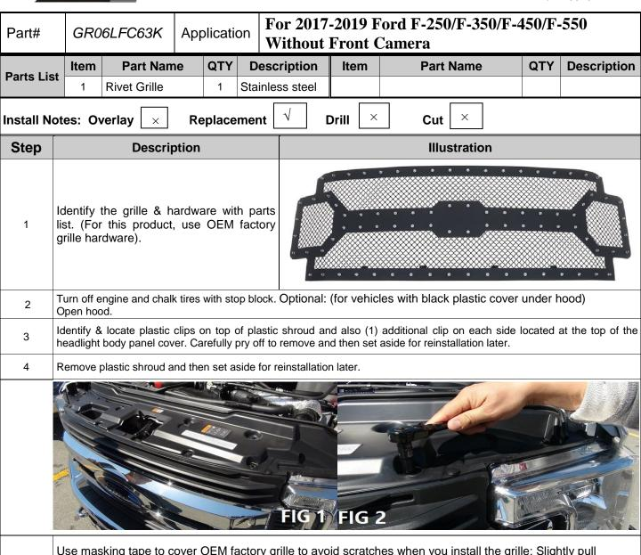
Use masking tape to cover OEM factory grille to avoid scratches when you install the grille; Slightly pull forward from top of the OEM factory grille (Fig 3). There are two clips (Fig 4) at the side of each corner. In order to remove the OEM grille shell, pull with more force at these two areas.
