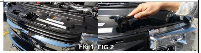
Use masking tape to cover OEM factory grille to avoid scratches when you install the grille; Slightly pull forward from top of the OEM factory grille (Fig 3). There are two clips (Fig 4) at the side of each corner. In order to remove the OEM grille shell, pull with more force at these two areas.
