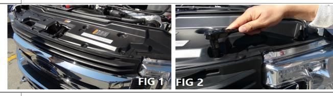
Use masking tape to cover OEM factory grille to avoid scratches when you install the grille; Slightly pull forward from top of the OEM factory grille (Fig 3). There are two clips (Fig 4) at the side of each corner. In order to remove the OEM grille shell, pull with more force at these two areas.
