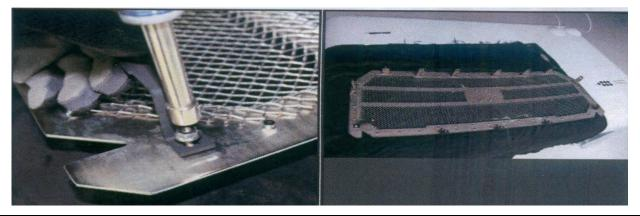
Reinstall shutter component to new Grille with factory hardware that was preciously removed.
