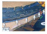
5.Remove Grille. Remove 6 Bolts on the Black Bar along the Bottom of. the Factory Grille and remove. (Fig. 4)
