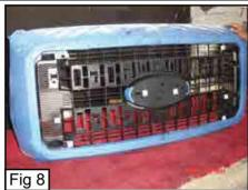
Now you need to cut out the inner section of the black grille section. You will cut around the inner edge of the black section as marked in (Fig 9). The 4 corner areas and the right and left sides will not be cut out, make sure to leave the areas marked in (Fig 10) attached to the black grille section on both the right and left sides. Sand all the cut areas smooth with a sanding wheel.
