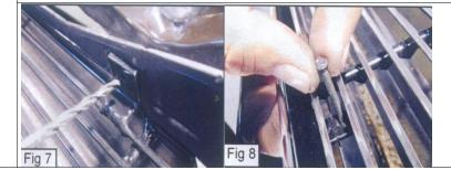
The instruction here is for your reference only. You may need to bend the billet grille bars or tabs a little bit to adjust to fit. We strongly recommend the professional installer for best result. Please use masking tape and tape the OEM grille shell along the edge to protect your vehicle during installation. We are not responsible for any damage caused by the installation. Thank you for choosing our product!
