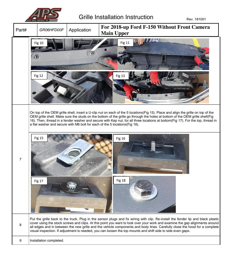
The instruction here is for your reference only. You may need to bend the billet grille bars or tabs a little bit to adjust to fit. We strongly recommend the professional installer for best result. Please use masking tape and tape the OEM grille shell along the edge to protect your vehicle during installation. We are not responsible for any damage caused by the installation. Thank you for choosing our product!
