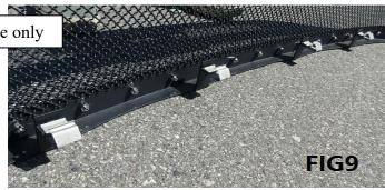
Carefully put back into place the headlight plastic body panel around the head lamp area making sure to align with tab fasteners and then firmly press into place. Use the bolts to mount and secure the panel on the inside wheel well lip.
