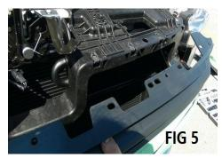
There are 4 metal clips near the bottom of the OEM factory grille shell; use your screwdriver and push slightly to release it. The OEM factory grille should now be free and ready to be removed. Carefully place the grille on a soft cushioned surface.
