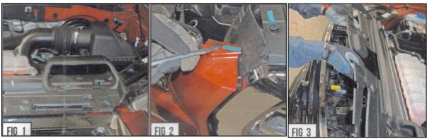
On the inside of the inner wheel well lip, remove (2) 7mm bolts. The headlight plastic body panel should now loose. You will need to coax panel out and off catch tabs to remove completely. The plastic wedge spatula should help.
