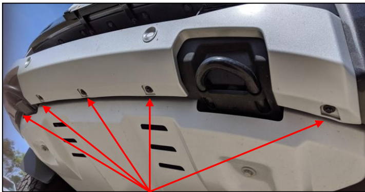
(Fig 1) Five Lower Valance Bolts
