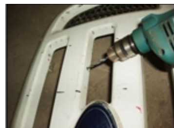
Figure 2 – Drill holes on the grille shell
