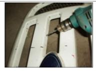
Figure 2 - Dill holes on the grille shell
