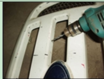
Figure 2 – Drill holes on the grille shell
