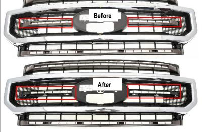
4 Install the U-clip nuts onto the tabs as shown.
