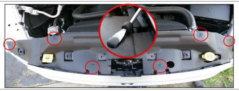
3 Using a 10mm socket, locate and remove 4 factory bolts securing factory grille onto vehicle. Set hardware aside for re-installation.
