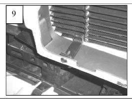
Connect the driving lights. Re-install the assembled bumper cover assembly back onto the vehicle. Make sure the signal light wires are in the bumper cover light holes. Carefully align the fender to bumper cover studs. Gently push the bumper cover in place. The three rivets from each wheel well splash shield are to be replaced with the plastic push-in retainers supplied in the hardware pack. Re-install the signal lights.
