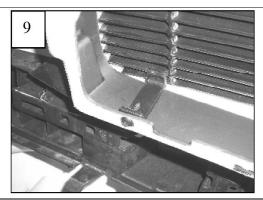
Connect the driving lights. Re-install the assembled bumper cover assembly back onto the vehicle. Make sure the signal light wires are in the bumper cover light holes. Carefully align the fender to bumper cover studs. Gently push the bumper cover in place. The three rivets from each wheel well splash shield are to be replaced with the plastic push-in retainers supplied in the hardware pack. Re-install the signal lights.
