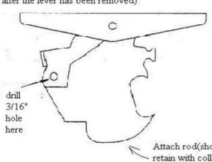
99-01 Dodge Dakota/Durango Hood safety release latch assembly illustration(looking at the back side of the latch assembly towards the front of the vehicle)
