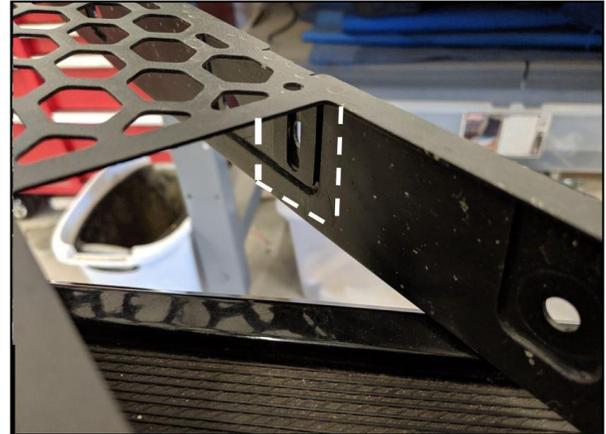
(Fig 6) Align Tabs With License Plate Holes
