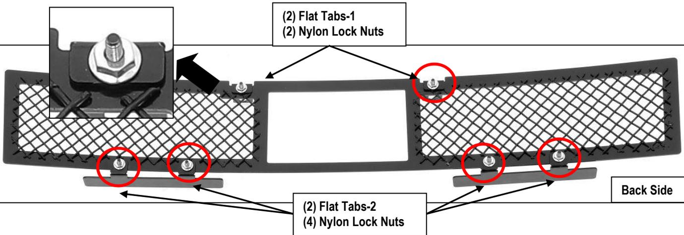
8 Remove the film from the Flat Tabs-2 on the grill insert, to install the grill insert onto the bumper valance. (Fig 5 & 6)
