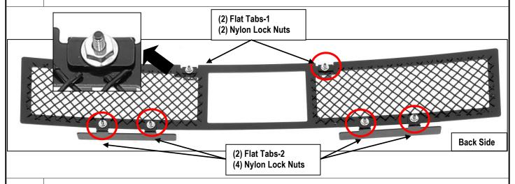
Remove the film from the Flat Tabs-2 on the grill insert, to install the grill insert onto the bumper valance.(Fig 5 & 6)
