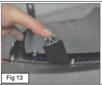
Put into place the (2)Brackets and using the (2)Flange Nuts, fix the Bracket to the new grille Replacement. There are (2) threaded studs that will Properly locate them into Position. Note Figure 16 for the correct orientation. (Fig 14-16)
