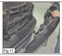
Take the new Grille Replacement and put into place the (2) Push Retainer Clips onto the grille's predetermined mounting tabs. (Fig 12-13)
