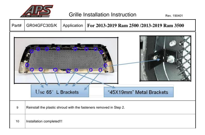
The instruction here is for your reference only. You may need to bend the billet grille bars or tabs a little bit to adjust to fit. We strongly recommend the professional installer for best result. Please use masking tape and tape the OEM grille shell along the edge to protect your vehicle during installation. We are not responsible for any damage caused by the installation. Thank you for choosing our product!
