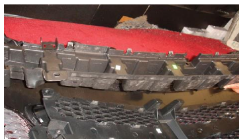
Step3-2:Remove Bumper Support.
