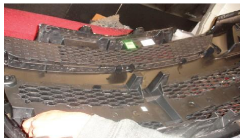
Step3-4: Remove Factory Grille.
